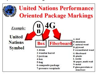
The markings on the outer container surfaces could be different for certain types of packages. All UN POP markings are permanently marked on the container. Handwritten marks are not authorized under the UN recommendations. The most common POP that is offered to FedEx Ground is the fiberboard box.
