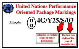
The last two digits indicate the year of manufacture. The number 03 indicate the package was manufactured and tested in 2003.
